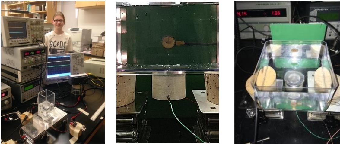
Figure 6. From left to right: Complete apparatus with levitation cell #1 and co-author KAH. Levitating bubble in tank appearing under transmitting transducer  $T_1$  in center of tank (due to side-view camera angle). Overview of levitation cell #2 looking downward with transmitting transducers  $T_1$  on north and  $T_2$  west tank walls, and the receiver on the southeast corner.
