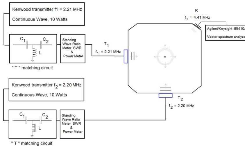
Figure 5. (On left): Schematic of cell #2 with supporting electronics and tank set-up for the nonlinear ultrasonic crossed beam scattering experiment in the presence of a single levitated bubble – detection at the sum frequency component 4.41 MHz.
