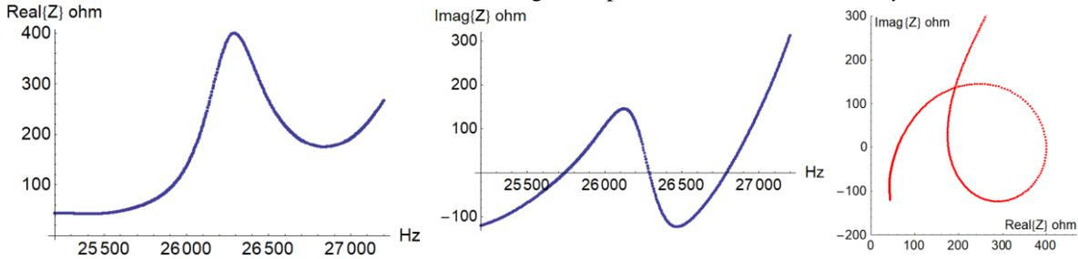
Figure 4. Left to Right: The real part and imaginary part of the electrical impedance  $Z$  of the cylindrical shell transducer vs. frequency; the circular impedance plot of the transducer (real  $\{Z\}$  vs. imaginary  $\{Z\}$ ).
