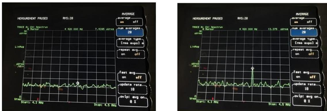
Figure 7. Received sum frequency component in the absence of a bubble in the interaction region. Received sum frequency component in the presence of a bubble in the interaction region. The transmitted primary frequency components are 2.21 and 2.20 MHz. The scattered sum frequency component is at  $f_+ = f_1 + f_2 = 4.41$  MHz. Horiz. Scale is 2 kHz/Div. Vert. scale is 3 micro Vrms/Div.
