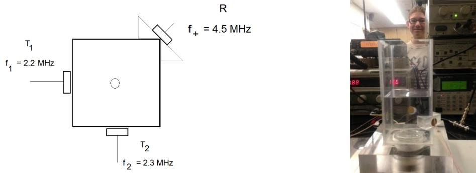
**Figure 1. Left to right: Top view of non-linear scattering setup of crossed ultrasonic beams in the presence of a levitated air bubble in water; combined acoustic cell levitation apparatus with crossed beam transmitting and receiving transducers, and co-author KAH.**
