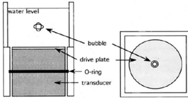
Figure 3. From Ref. 3, diagram of levitator in side and top views showing mounted transducer and water filled chamber. A bubble is illustrated at the approximate levitation position undergoing axisymmetric quadruple shape oscillations. The base of the open tank is 3 in. x 3 in. and the transducer height is also 3 in.
