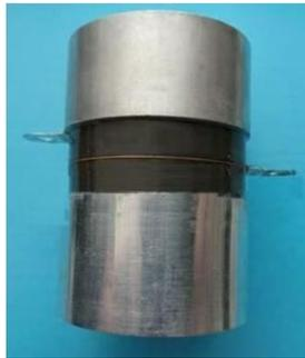
*Figure 4. A commercially available Langevin ultrasonic transducer model SMLTF120W60 used in Figure 3 above. A sandwich transducer is often called a Tonpilz transducer – meaning a singing mushroom.*
