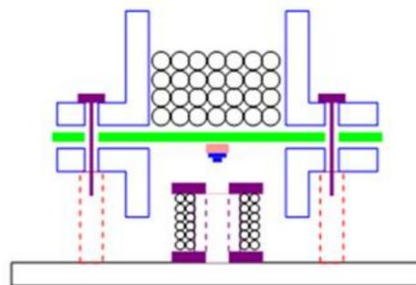
Figure 2. Cross-section of the Soil Plate Oscillator (SPO), that is driven from underneath the clamped acrylic plate by a swept sinusoidal signal going to the AC coil. This drives the magnet with the accelerometer attached to measure the frequency response. Drawing by Emily Santos.
