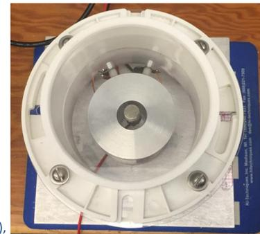
Figure 3. A 4.5 inch diam SPO made from PVC flanges and a 1/8 inch thick acrylic circular clamped plate. AC coil, rare earth magnets and accelerometer is on underside of plate.
