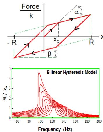
A bilinear hysteresis model can be used to predict the nonlinear tuning curve upward curvature behavior. See Ref. 1.
