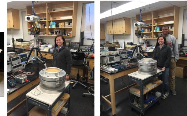
Figure 5. The 8 inch diam SPO is filled with 3440 grams of sifted masonry sand. The clamped plate mass is 108 grams. The SPO can be driven from the underside by a swept sinusoidal amplified current going to AC coil. The coil field drives the rare earth magnets located on the underside of the 1/8 inch thick acrylic plate. The accelerometer fastened to the magnet (1 cm in diam) generates a response signal that goes into a charge amplifier and then to the Agilent 35670A dynamic spectrum analyzer.
