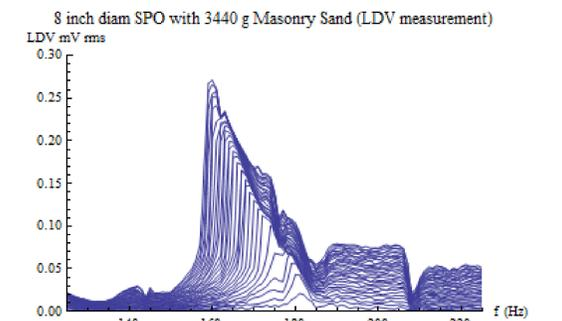
Figure 6. Nonlinear tuning curve response off the sand surface vibration on axis. Notice the linear backbone peak ridge.
