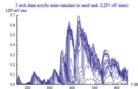
Figure 9. LDV surface velocity measurement for “on the target” and “off the target” particle velocity response vs. frequency. The mine is 1.5 inches in radius, and has a height of 2 inches. The “off target” location is at the position  $x = -4.5$  inches from the center. The concrete soil box is 12 inches by 12 inches by 3.5 inches deep.
