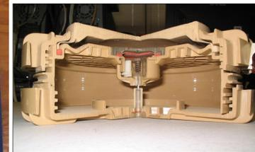
Figure 4. Cross-section of VS - 1.6 plastic “inert” landmine, 8.5 inch diam by 3.5 inches in height.
