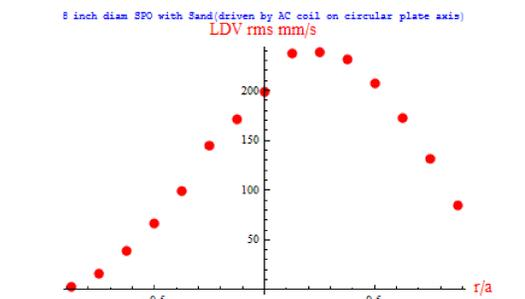
Figure 7. The LDV response near 160 Hz across the sand surface.
