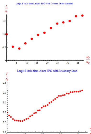
Figure 8. The normalized resonant frequency vs. (A) 10 mm glass bead loading or (B) masonry sand loading exhibits first a decrease in resonant frequency followed by a notable increase. This is due to the elastic “disk” layer of the granular medium having a more dominant increase in its effective lumped spring constant K [which is proportional to the cube of its thickness (or mass) ] while the granular mass loading increases linearly. The plate mass is  $M_p = 108$  grams.
