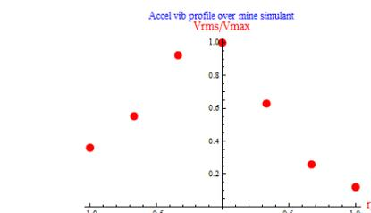
Figure 10. Accelerometer vibration measurement of the sand over the 1.5 inch radius buried acrylic mine simulant (in the soil box). Measurement taken near 300 Hz.
